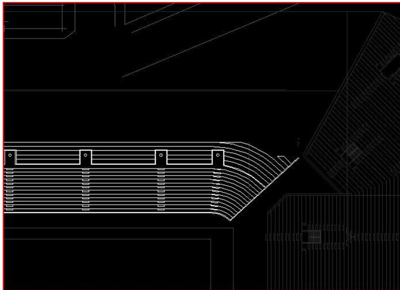
Fig 11. Lower Bullens/Paddock plan View, showing new vomitories arranged around support columns.
