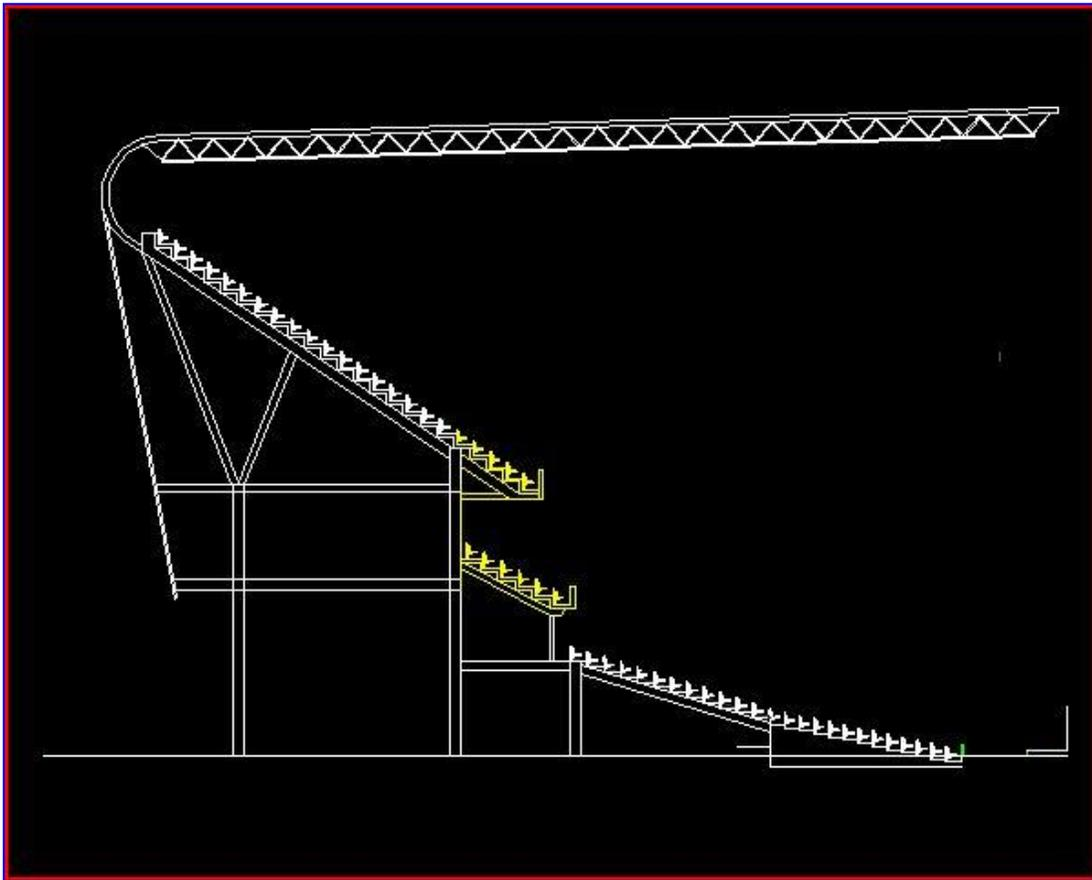
**Fig 15. New upper tier with new Exec tier inserted.**
