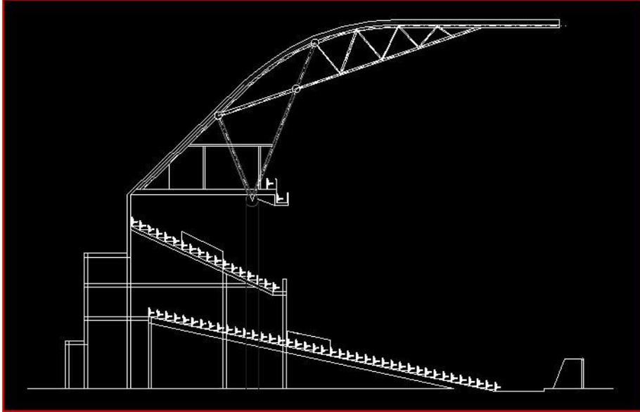
**Fig 21a** New Gwladys Street stand with 'Skyboxes' built into roof-truss.
