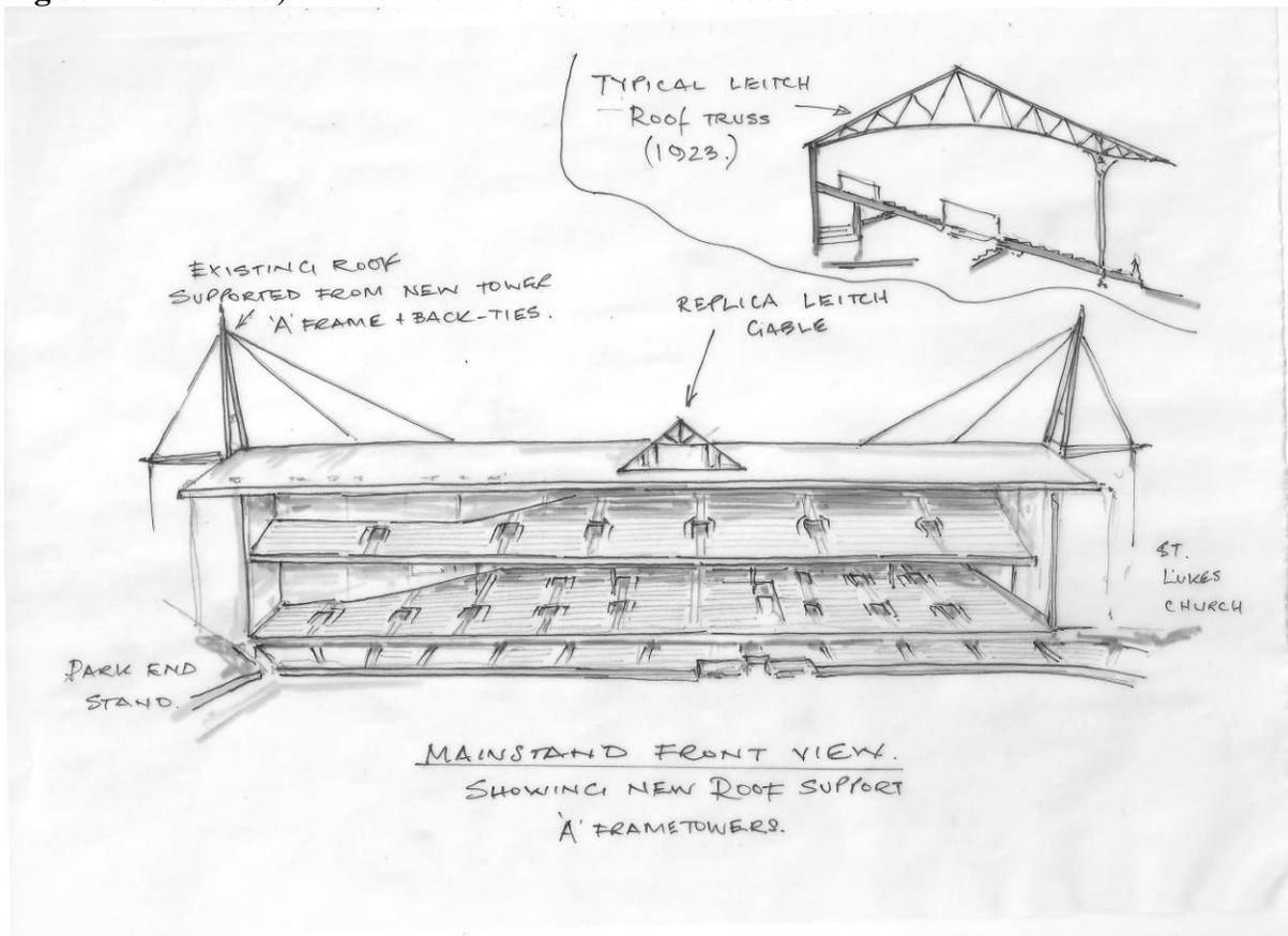
**Fig 31. Mainstand with front roof supports removed and back-stays supporting existing segmented roof truss With Replica Leitch Gable on the centre-line.**
