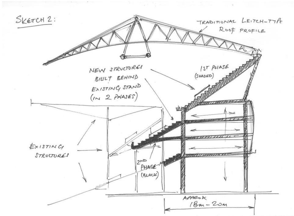
Above: Fig 19. Cross section of new two-tiered Bullens Rd Stand Extension.
