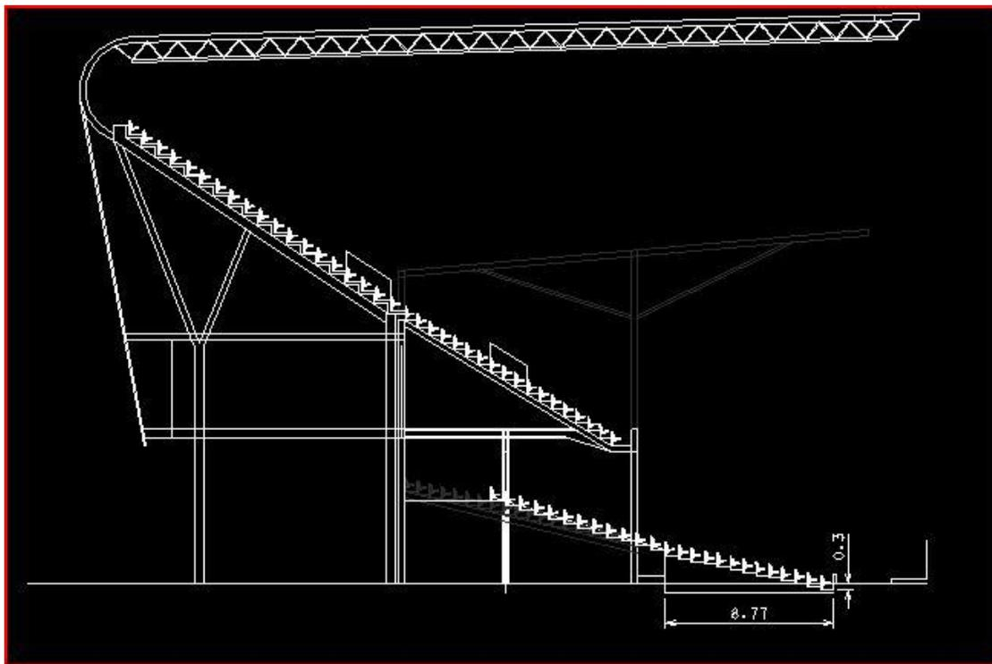
Fig 13. Extended upper tier. Note existing roof shown in grey (Roof Truss not shown)
