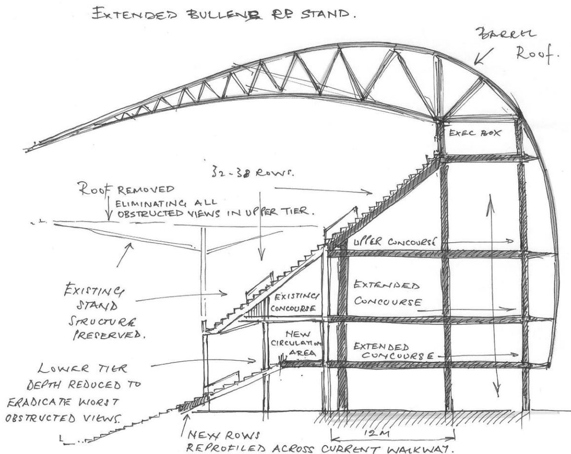
**Fig 16. Extended Bullens Rd stand Cross section.**
