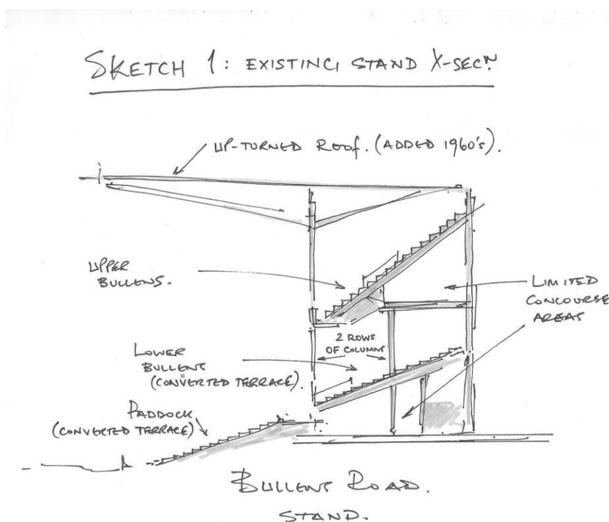
**Fig 8. Bullens X-Section**
