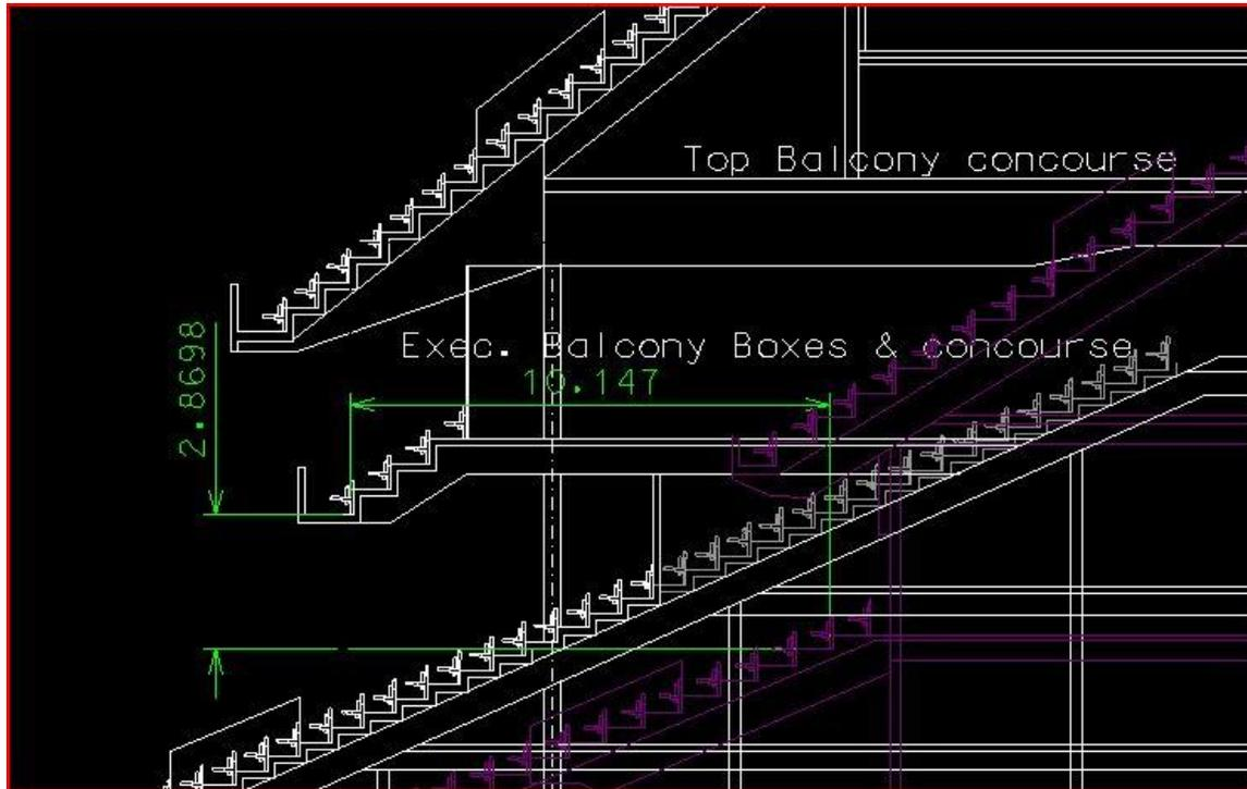
**Fig 52. Comparison between Exec box positioning. (Kirkby shown in purple)**
