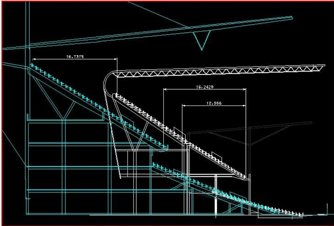
**Fig 51. Comparison: Kirkby cross-section superimposed on extended Bullens Rd stand.**
