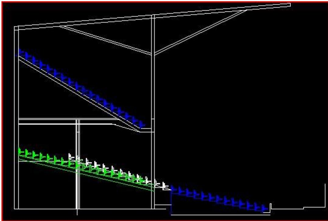
**Fig 9. Re-profiled Lower Bulls (green seats are replaced by those shown in white.)**
