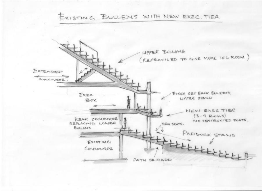
**Fig. 12a: Perspective view of Bullens Rd Stand with Exec deck beneath an extended upper tier. (Inset Fig 12b: Existing Bullens)**
